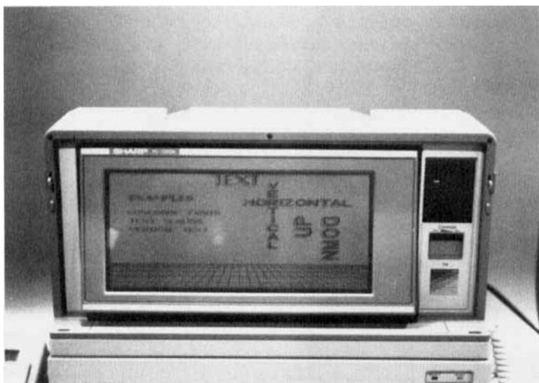
FIGURE 5 Supertwisted LCD in transportable computer with backlighting. See Color Plate V.
